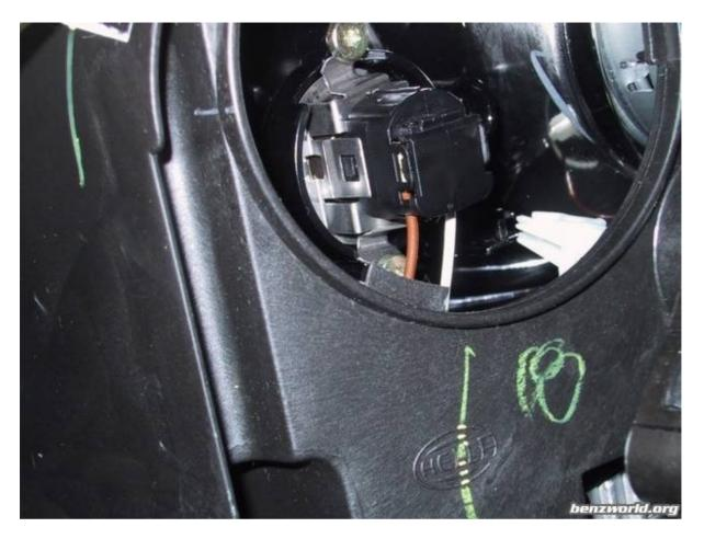
3) Trace the wires above from the halogen bulb to just under the Xenon bulb. You will need to carefully use the needle nose pliers to pull both wires out further so that you can access them. See picture below.
