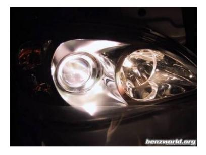
This modification will allow the N.American flash-to-pass halogens to activate with the Xenon high beams just as the E-code (European code) Bi-Xenon lamps do.
